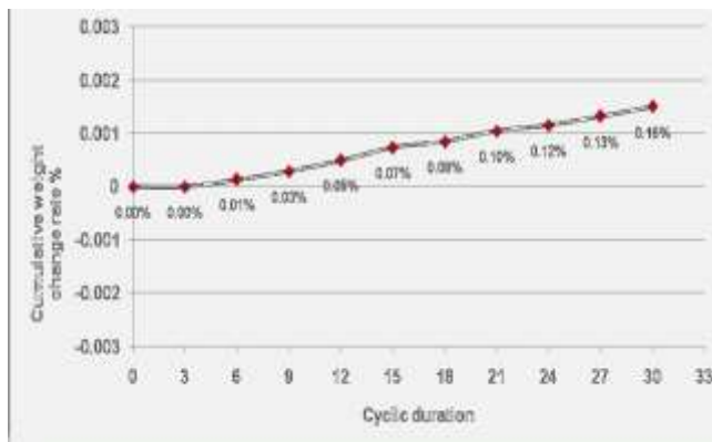
Fig 6.5(a) Weight loss of specimen under HCL attack
